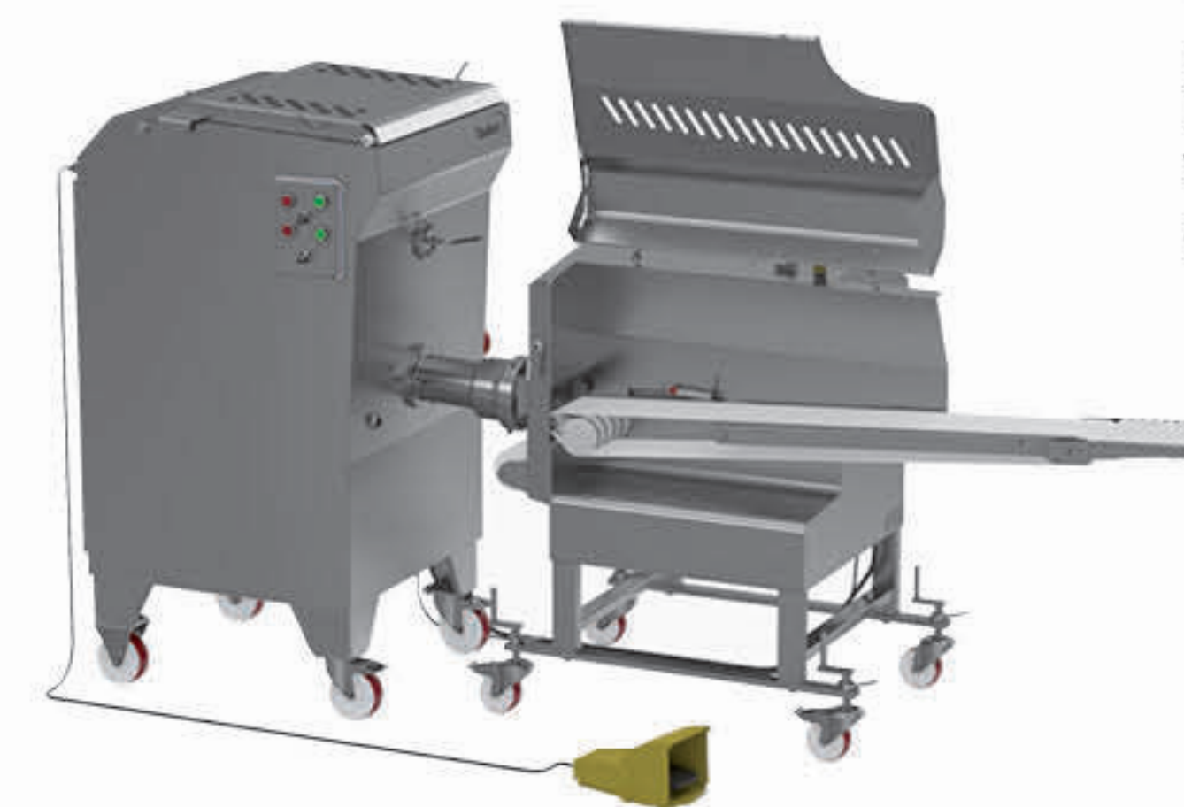
Raccordement TX32ML + Portio 140 Connecting TX32 ML + Portio 140
